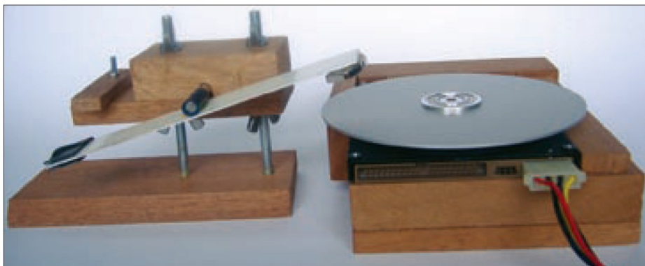
Fig. 1. Levitation of a magnet over the rotating aluminum disk.
